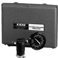
KIENE Peak Pressure Indicators Model K-100 (0-140 bar) Model K-107 (0-210 bar) Model K-108 (0-250 bar)
